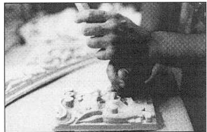
FIGURE 7: The wood carver creates a new master pattern. A good pattern design will compensate for metal shrinkage.
