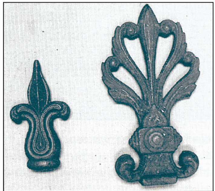
FIGURE 8: These two iron finials were originally cast in Ohio during the late 1800's. To reproduce these, an epoxy mold was made, and the resulting finial was re detailed.
