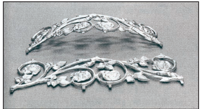
FIGURE 1: This rose panel can be bent 3 inches without cracking.
