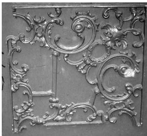
Fig. 2: Above, these designs were fabricated "loose" to save on the cost of permanent tooling.
