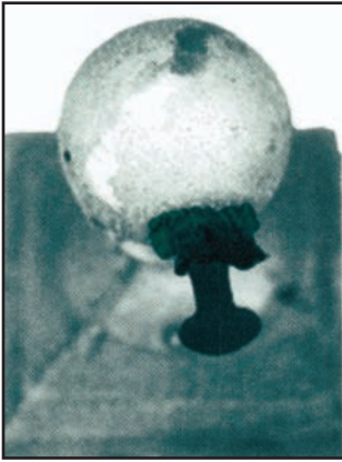
Left: Dissimilar metals in almost any form can cause severe corrosion. The green area shows severe galvanic corrosion caused by a marine-grade aluminum ball cap attached to a stainless steel bolt.
