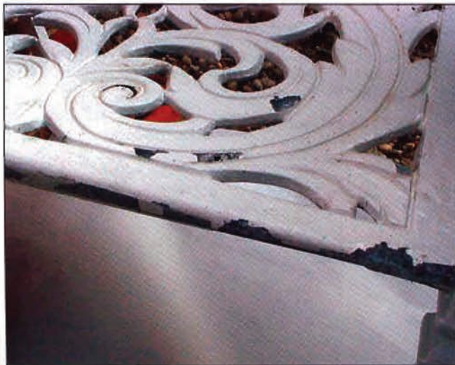
This 12-year-old aluminum furniture in Dallas, TX, is also not marine grade. Even though it is not in a harsh marine environment, its powder coat is peeling and corrosion appears.
